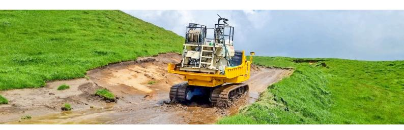
Although we were able to access majority of areas with our 4x4, 6x6 and 8x8 trucks, in the early stages to access certain areas we mobilized a Marooka tracked machine and mounted one of our smaller hydroseed units onto it. This meant we could still stabilize sites that were only accessible by tracked machine, which was extremely helpful to our client and showed our commitment to completing the project in full and on time.
